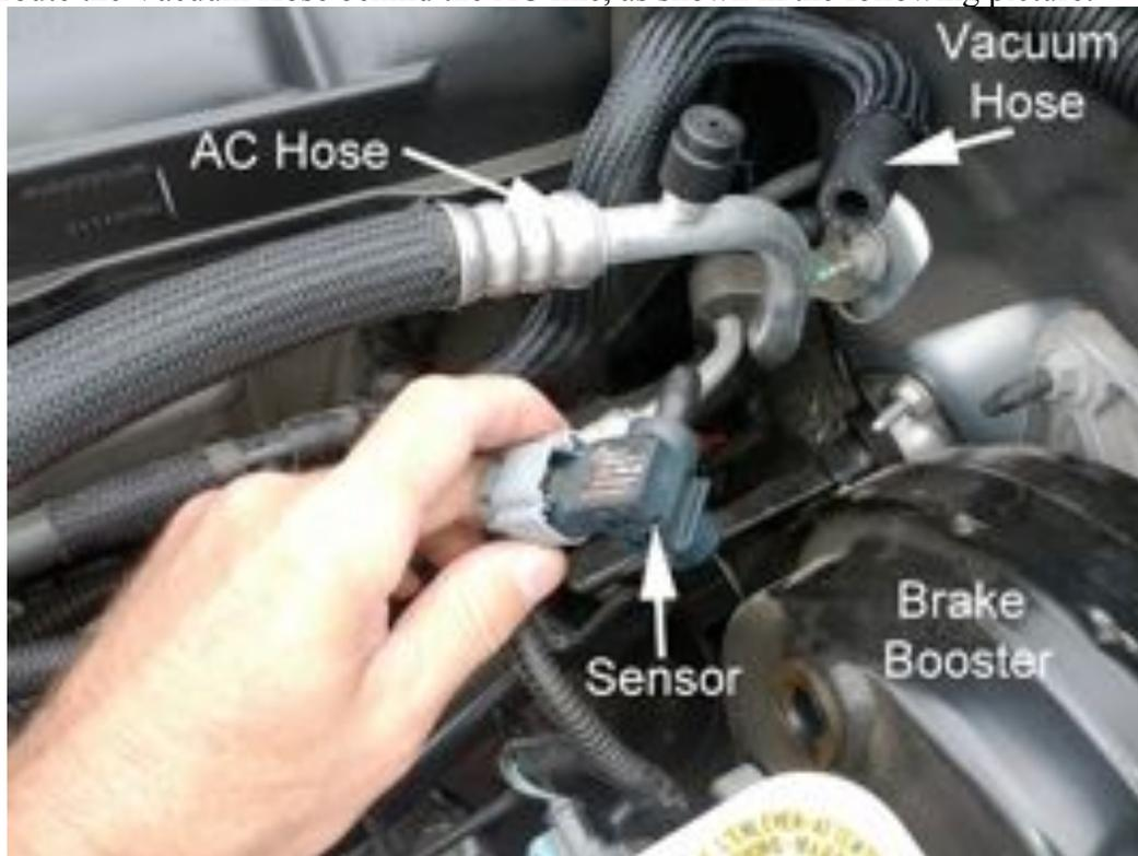
3. Insert the 90 degree plastic fitting (attached to small hose) into the brake booster. You'll have to press hard, but it will go.
