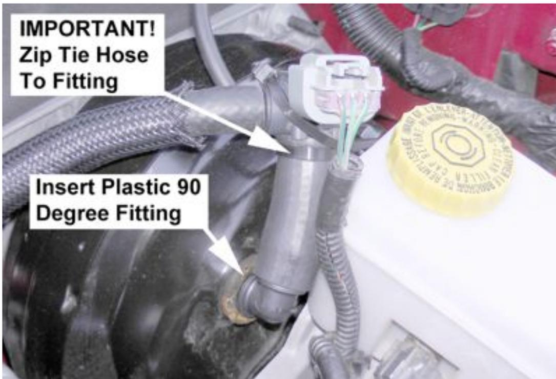
6. Zip tie the sensor to hold the hose clear of the compressor head.
