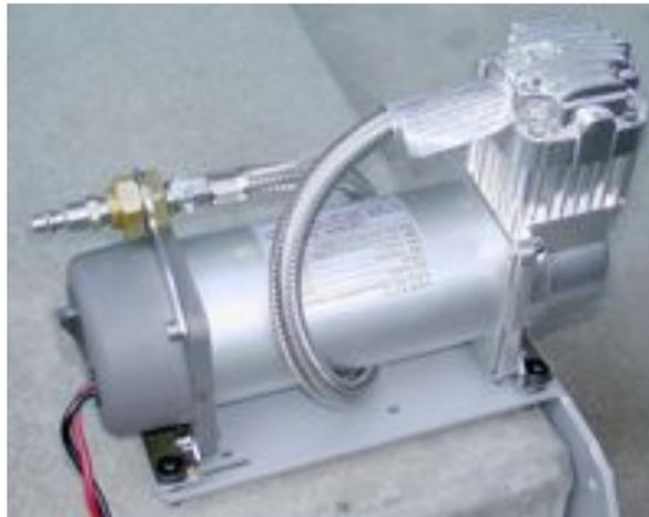
Use thread sealant for proper installation. Teflon tape is not recommended. Properly sealed, recommended torque is 12 to 15 ft. lbs.
