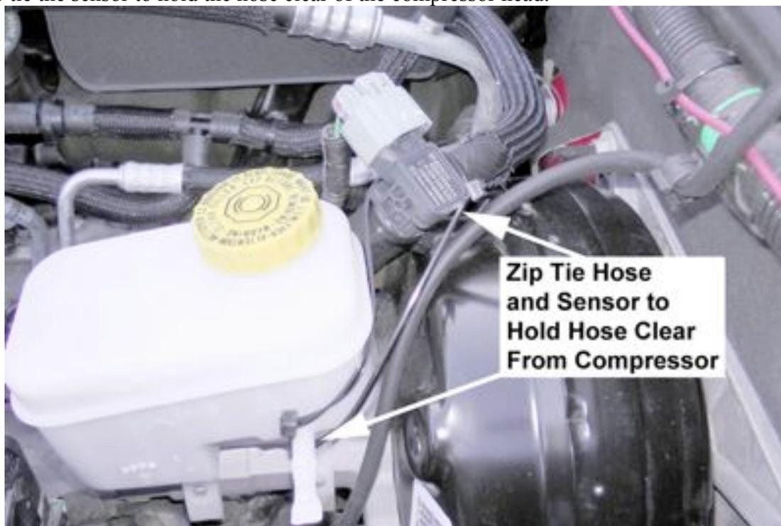
7. Install the compressor and bracket assembly onto the master cylinder studs and run power and ground wires.
